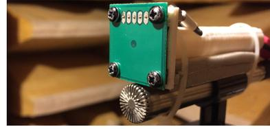
Figure 2. DUT and SLM microphones mounted
