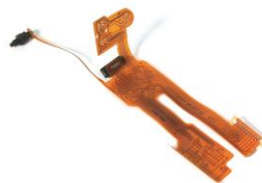
The flex circuit solution: A single circuit with 7 stiffeners and 2 connectors provides all the needed interconnects.
