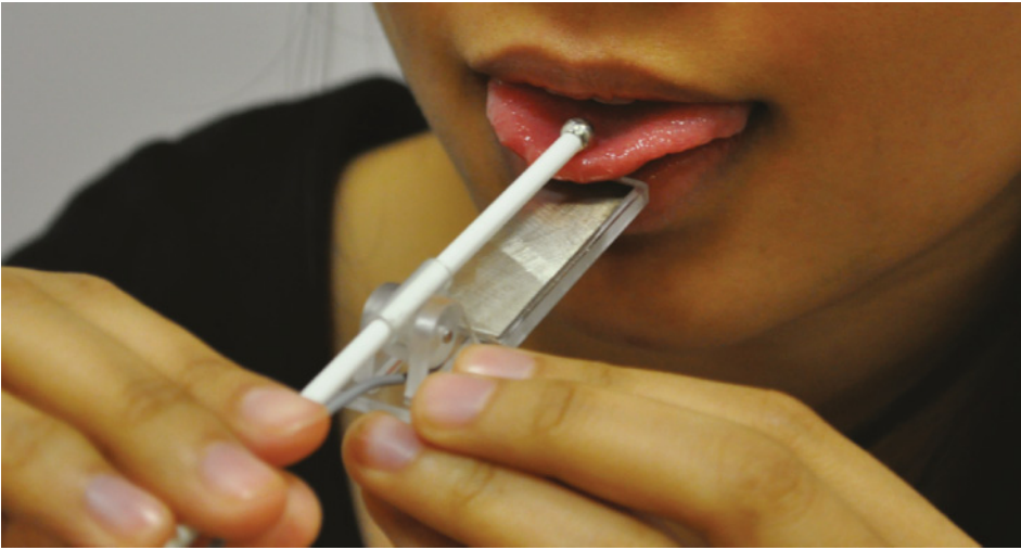
Fig. 7. A close-up of the tongue interface that connects with the participant's tongue.
