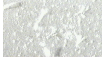
Heterogeneous nature of rosin based flux medium with evidence of rapid crystal formulation.
