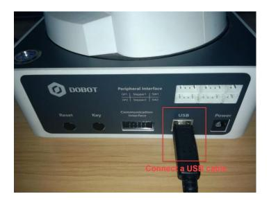
Figure 2.2 Connect the Dobot Magician to your computer
