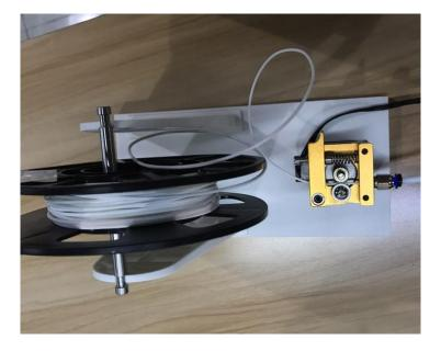
Step 7 Place the filament and the extruder to the filament holder, as shown in Figure 5.125.
