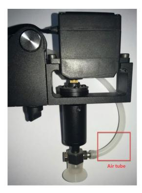
Figure 5.9 Install an air tube
