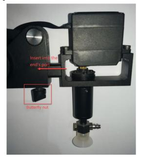
Figure 5.8 Install a suction cup kit
