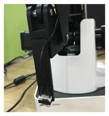
Figure 5.170 Fix auto-levelling tool
