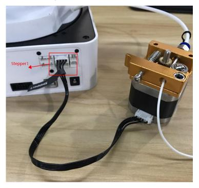
Figure 5.124 Connect with extruder
