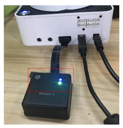
About 5 seconds later, the green LED indicator on the WIFI module is on, indicating that the Dobot Magician has been connected with WLAN, as shown in Figure 5.179.
