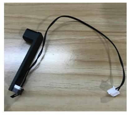
Figure 5.169 Auto-levelling tool
