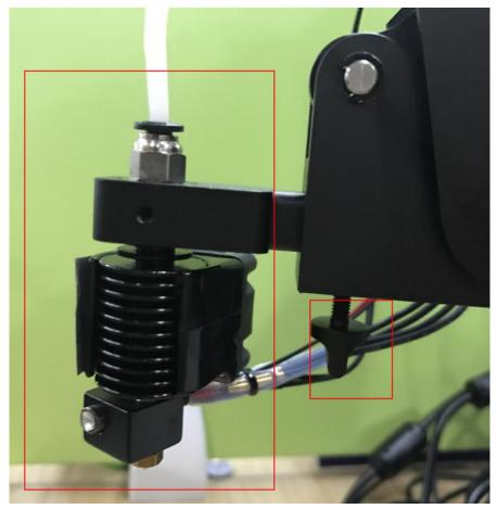
**Step 4** Fix the hot end on the Dobot Magician with clamp fixing screw, as shown in Figure 5.122.
