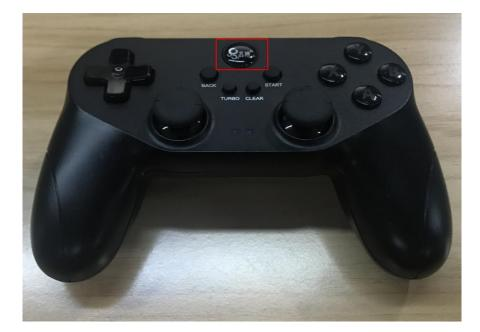
Figure 5.187 Power button of the stick controller
