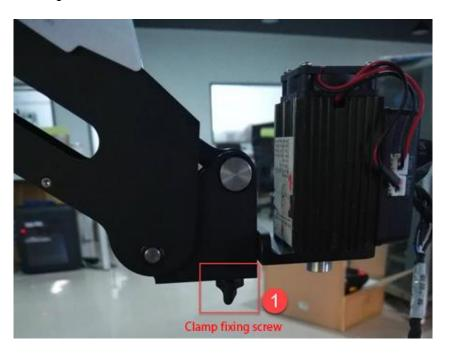
Figure 5.60 Fasten the laser with clamp fixing screw
