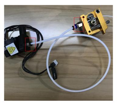
Figure 5.121 Connect extruder and hot end
