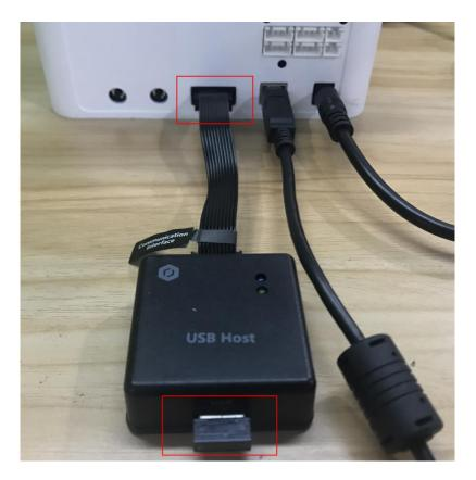
Figure 5.186 Connect with USB Host module
